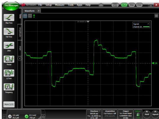
Figure 4. De-emphasis capability is built into the M8062A, not requiring external signal processing boxes which add cables and complicate the test set-up
